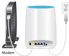
Unplug your modem and remove and replace the backup battery if it uses one. Plug the modem back in.
